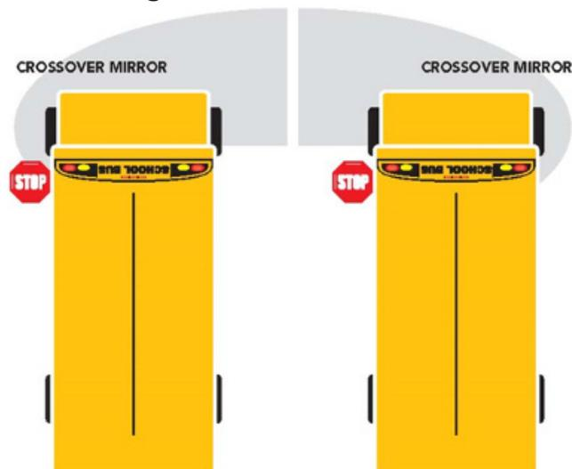
Figure 3.5 illustrates how the left and right side crossover mirrors should be adjusted. This would include cones A-K in the Federal Field of View Test. See Federal Field of View Illustration.
